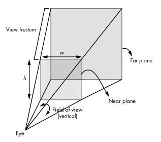
Figure 9-5: Perspective projection camera model
