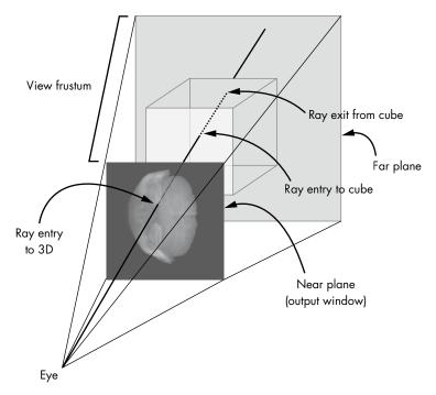
Figure 11-2: Perspective projection of 3D volumetric data
