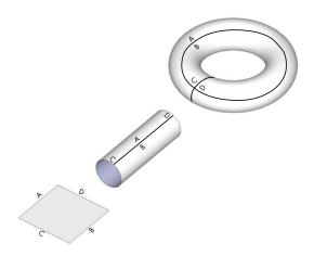
Figure 3-2: Conceptual visualization of toroidal boundary conditions
