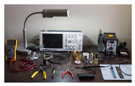
Figure B-2: A typical electronics workbench, with a multimeter, a task lamp, clamps, a wire stripper, a screwdriver, needle-nose pliers, a loupe, solder, flux, an oscilloscope, and a soldering station.
