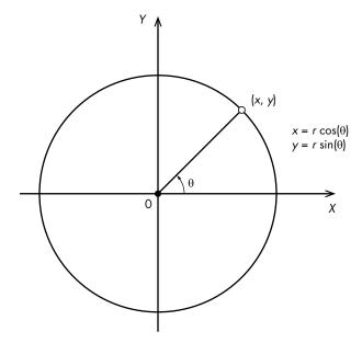
Figure 2-2: Describing a circle with a parametric equation
