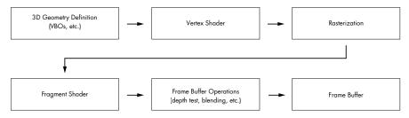
Figure 9-3: The (simplified) OpenGL graphics pipeline
