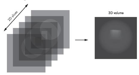
Figure 11-1: Building 3D volumetric data from 2D slices
