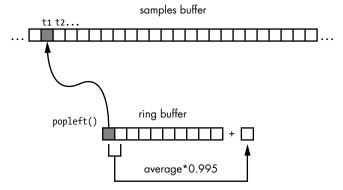
Figure 4-3: Ring buffer and the Karplus-Strong algorithm
