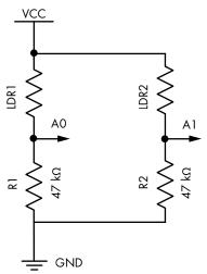
Figure 12-4: Schematic of a simple light-sensing circuit
