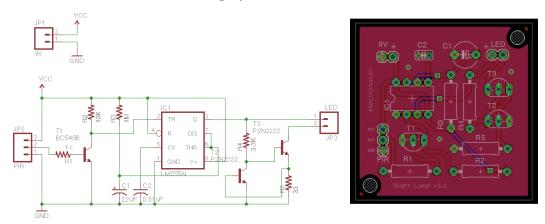
Figure B-4: A circuit schematic and the matching PCB design created with EAGLE
