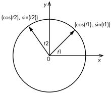
Figure 5-1: Generating random unit velocity vectors
