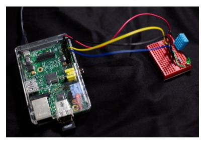
Figure 14-6: The Raspberry Pi, DHT11, and LED connected with a breadboard
