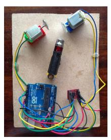
Figure 13-9: The completely wired laser display
