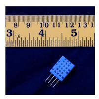
Figure 14-1: The DHT11 temperature and humidity sensor
