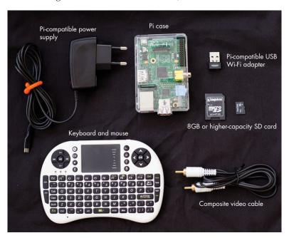
Figure 14-3: Recommended set of Raspberry Pi peripherals
