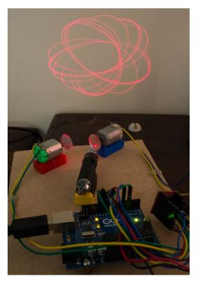
Figure 13-10: The complete wiring of the laser display and a pattern projected on the wall
