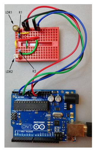
Figure 12-1: A simple light-dependent resistor (LDR) circuit assembled on a breadboard and connected to an Arduino Uno
