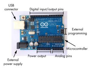
Figure 12-2: Components of the Arduino Uno board
