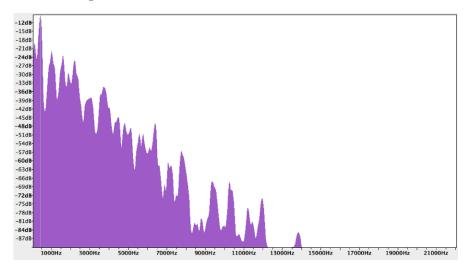
Figure 4-2: Spectral plot of note D4 played on guitar
