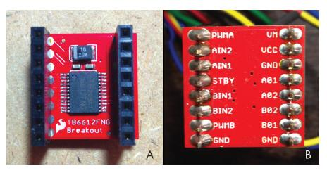
Figure 13-3: SparkFun Motor Driver 1A Dual TB6612FNG
